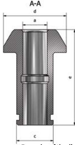
Examples of the dimensions of single-stage rotary coupling sleeves with two inner stages
